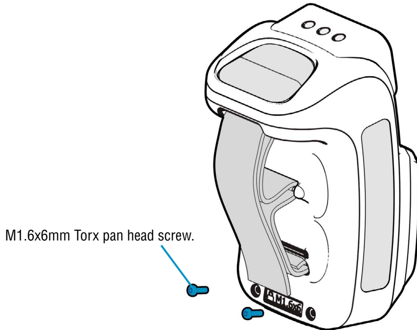
FIGURE 10: Battery cover locking screw location
